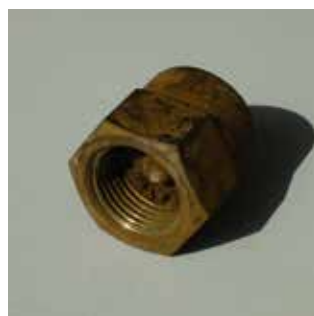
Clogged vane of a full cone nozzle
