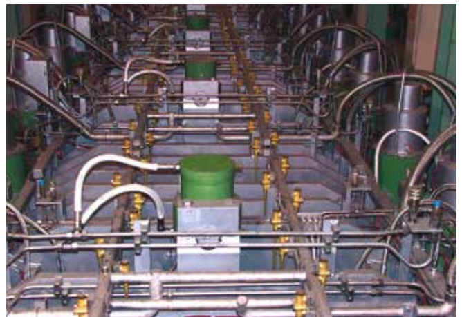
Horizontal segments with Mastercooler SMART nozzles
