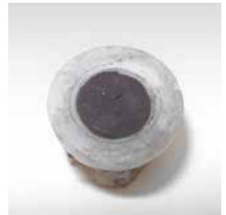
Clogged nozzle (back side)
