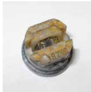
Clogged nozzle (front side)
