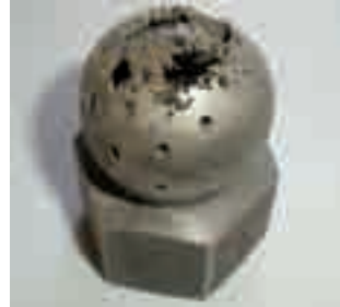
Fig. 1: Chemical corrosion of a spray ball
