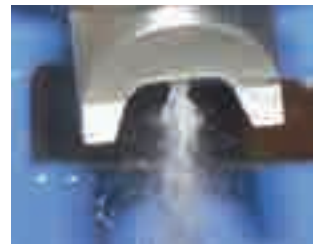
Figure 11: Atomization of gelatine with a Lechler ViscoMist twin-fluid nozzle
