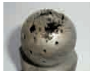
Figure 10: Chemical attack on a spray ball
